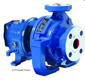
Center line mounted in a heavy duty fabricated steel casing support, the Model HT 3196 minimizes shaft misalignment and piping strain associated with elevated temperatures up to 700° F. As a member of the ANSI pump family the HT3196 features Goulds Pumps' premier i-FRAMETM power end, multiple seal chamber options including the TaperBore PLUS, and a wide variety of rigid and rugged mounting systems.
